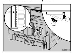
Attach the back plate to its original position.
