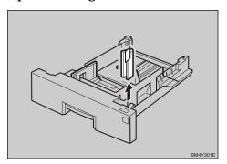
While lifting the front of the paper tray, place it into the printer. Then slide it into the printer until it stops.
