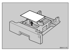
**7** Remove the red protective sheet taped on the guide.
