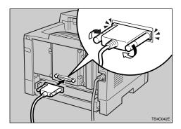
**1** Attach the other end of the cable to the interface connector of the computer.
