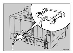
**1** Attach the other end of the cable to the interface connector of the computer.
