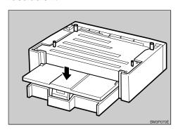
There are four pins on the top of the paper feed unit that point straight up. On the bottom of the printer, there are four holes. Align the holes over the pins and lower the printer gently onto the paper feed unit.
